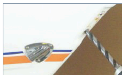
Ream out the holes to 12mm (0.475"), preferably with a 12mm drill size
