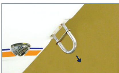
Removing the U-bolt
