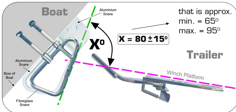
The ‘Latch Support’ can be mounted at an angle using the ‘Wedge’ side plates. This provides a simple way of adjusting the angle (X) that exists when the Latch hits the Snare.
