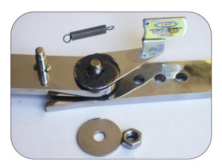
You must grease all contacting parts on assembly. Stainless steel will 'bind' badly if you do not lubricate.
